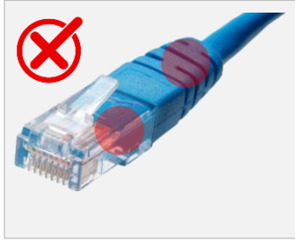
Plastic shielding is not compatible with PoE
