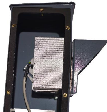
Nanopak5 LPR unit, already mounted inside of the totem on a swiveling bracket.
